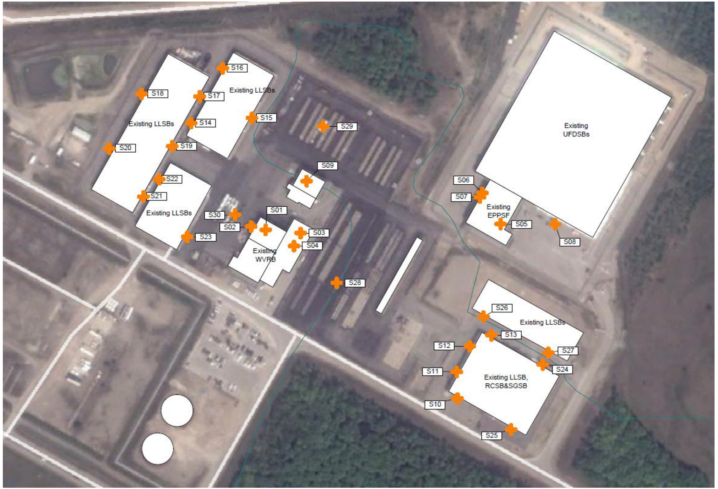
Figure 3-5: WWMF Significant Noise Source Locations 20
